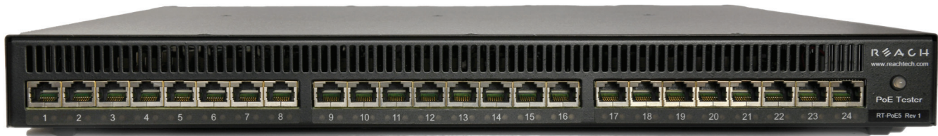
The PoE5 is in a 1U enclosure with 24 ports
